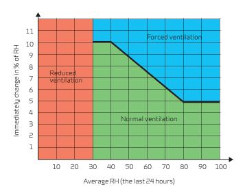
If the air humidity changes by more than 5-10% in relation to the average level, the unit responds with a higher rate of air exchange accordingly.
